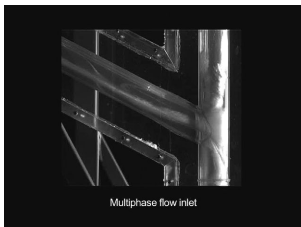
Figure 2. Flow visualization of the inlet separation region.
